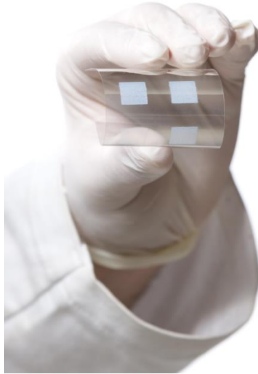
Figure 18. TiO 2 /SiO 2 hybrid nanocomposite flexible photoanodes inkjet-printed onto ITO/PET foil, taken from Ref. 7 .
